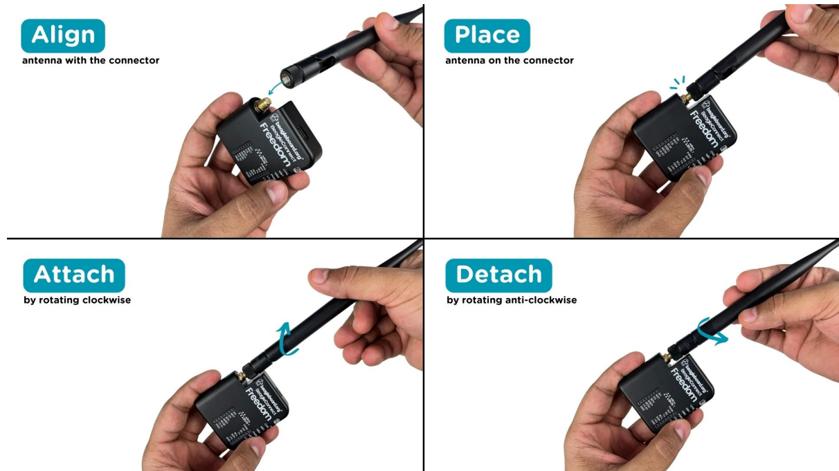
Fig. 12.1: Attaching antenna to BeagleConnect Freedom
